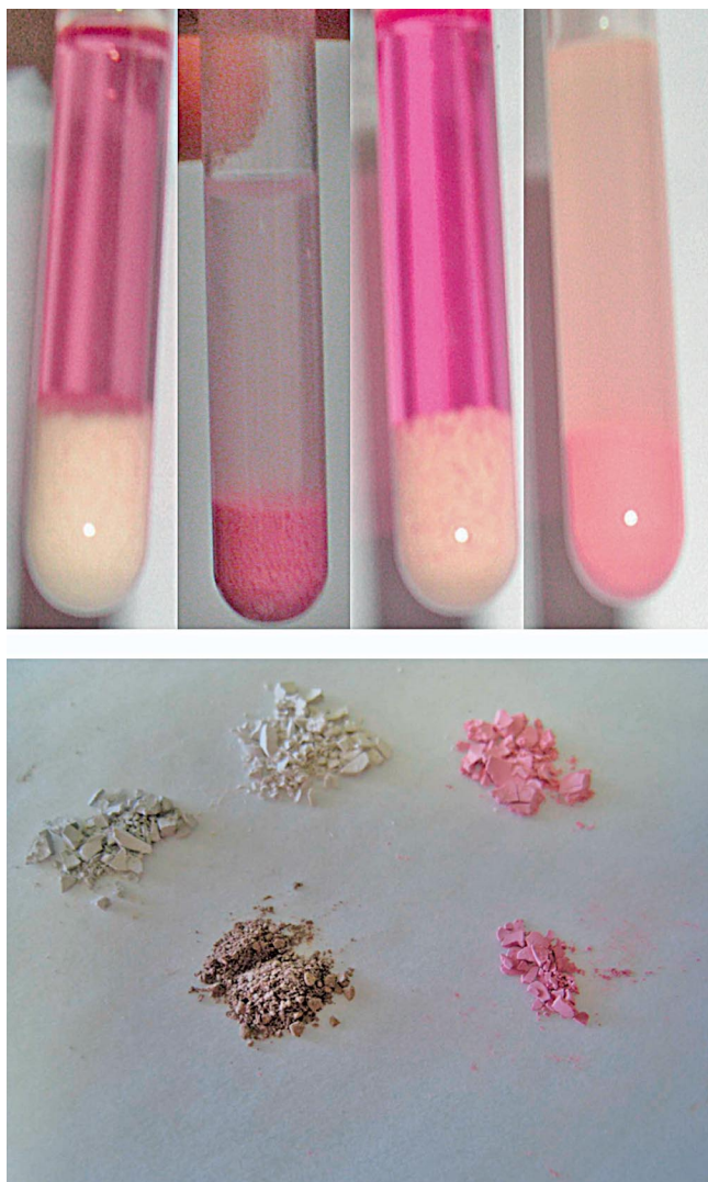
Figure 4. (Top) Slurries of TiO 2 nanoparticles with left to right: tpp, (tpp)Zr(OAc) 2 , Zn(tpp), and (tpp)Hf(OAc) 2 . 30 mg of TiO 2 nanoparticles were treated with 0.5 mM porphyrin solution (2 mL) by mixing slurry overnight, removing the solvent, and rinsing with toluene (2 or 3 times). (Bottom) Powders on upper row from left: tpp, Zn(tpp), and (tpp)Zr(OAc) 2 ; lower row from left: tpp (thf used as solvent and for rinse) and (tpp)Hf(OAc) 2 .
